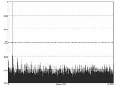
The plot below shows a 16384 point FFT plot of a 1 MHz tone sampled at 50 MS/s using a Blackman window.
